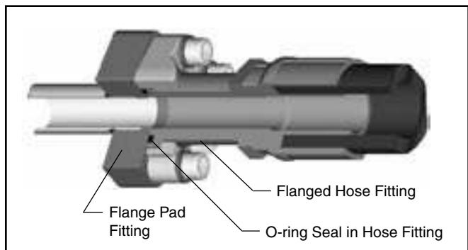
Fig. M1 – Flange Pad Fitting
