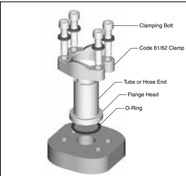
**Fig. M3 – Four-Bolt Flange Connection (SAE J518)**
