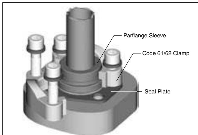
Fig. M2 – Assembly / Removal SAE J518 Connection
