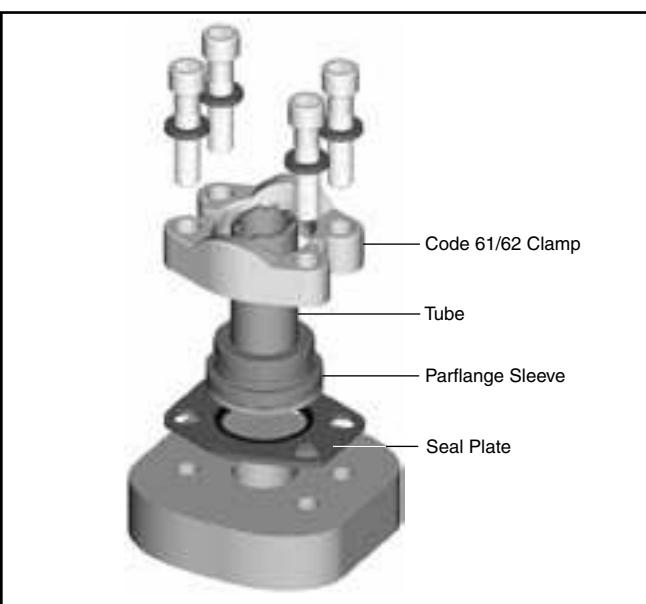
**Fig. M4 – Formed Tube with ISO 6162 (SAE J518) Connection**
