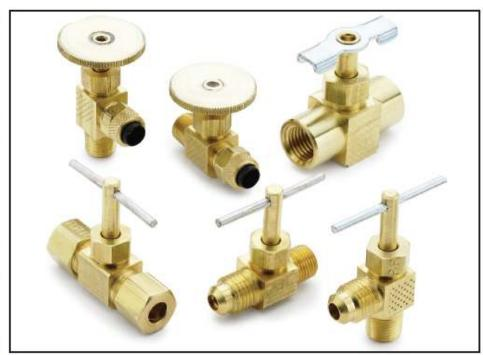
Needle and truck valves have metal-to-metal seats with fine thread screwdown. The lanyard valves' compact design is ideally suited for releasing condensate from air tanks. Brass construction with specially formulated low temperature seal which remains elastic to temperature as low -40°F.
